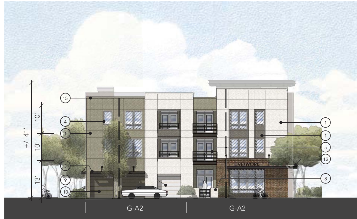
2. GARAGE SIDE ELEVATION
